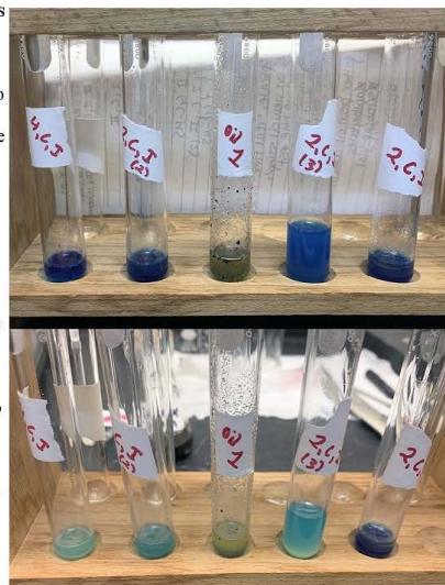
Figure 2. Methylene blue test results from Day 0 (top) and Day 5 (bottom).
